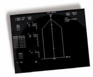
Where multiple antennas are installed, different position offsets for each antenna in the radar system should be applied with respect to the CCRP. If you switch between scanners (up to 8 possible - option), the information displayed is generated, which allow for consistency and uniform output.
