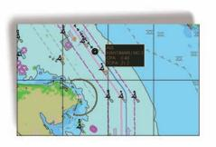
Also, it is easy to activate, deactivate and switch between AIS target symbols. This simply can be done with an integrated AIS filter, prioritising the targets within a dedicated area.
